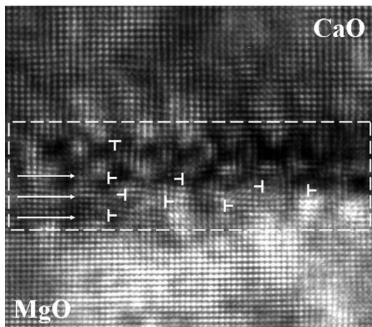
FIG. 3. Cross-sectional HRTEM image of the interfacial structure between CaO buffer layer and MgO substrate.
