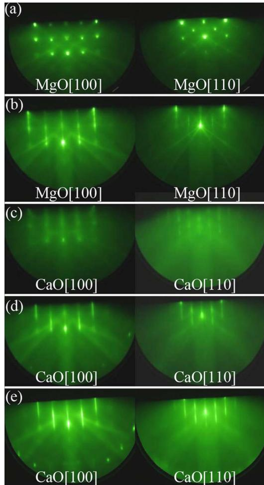
FIG. 1. (Color online) RHEED patterns taken during growth of a CaO film. The patterns are observed on  $\langle 100 \rangle$  and  $\langle 110 \rangle$  azimuths of the MgO substrate; (a) the MgO substrate after chemical polishing showing a spotty pattern, (b) the homoepitaxial MgO layer, (c) the nucleation of a CaO layer after several seconds of growth, (d) as-grown LT CaO buffer, and (e) as-grown HT CaO epilayer.
