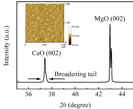
FIG. 2. (Color online) XRD ( $\theta$ - $2\theta$  scan) from the (002) peaks of CaO and MgO. The inset shows the AFM image of an as-deposited CaO surface (rms roughness: 1.2 nm, in a scale of  $2 \times 2 \mu\text{m}^2$ ).
